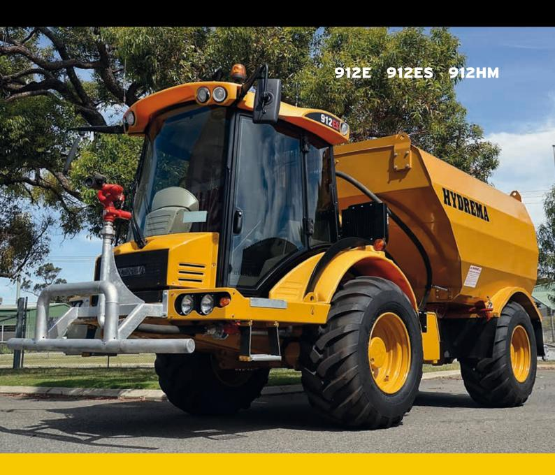
A unique combination of articulated center pivot, wide wheels and high ground clearance. For high mobility and low ground pressure.
